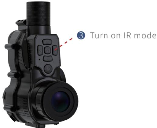
Turn on the IR mode, press and hold the "+" key, the picture will turn black and white, that is, the IR mode has been turned on, and then press and hold again to switch the first, second and third gear of IR and close. They are respectively weak, medium and strong gears. In order to save power, the weak gear can be seen clearly, so the medium and strong gears are not needed. Use color mode to view directly in daytime and light environment.
