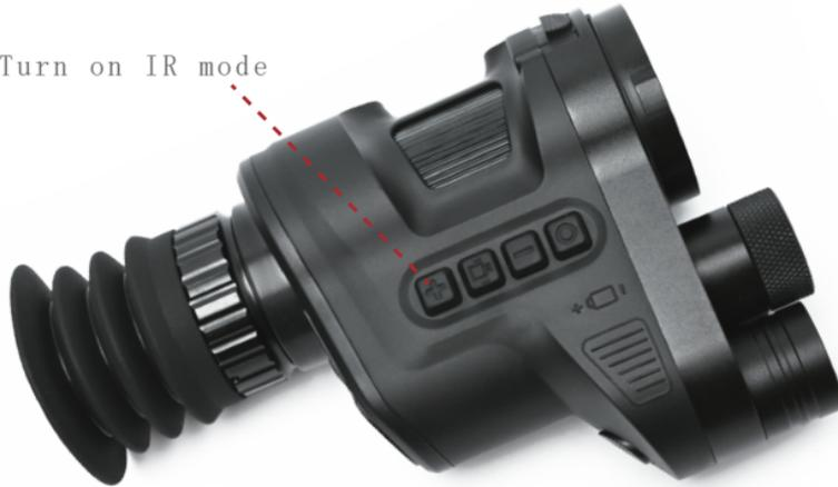
Turn on the IR mode, press and hold the "+" key, the picture will turn black and white, that is, the IR mode has been turned on, and then press and hold again to switch the first, second and third gear of IR and close. They are respectively weak, medium and strong gears. In order to save power, the weak gear can be seen clearly, so the medium and strong gears are not needed. Use color mode to view directly in daytime and light environment.
