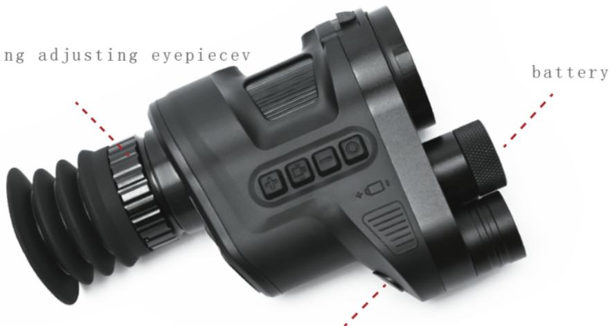
1、The diopter adjustment only needs to be adjusted once when the same person uses it. It is to adjust the degree of the eyes and the display screen, which has nothing to do with the picture viewed.
